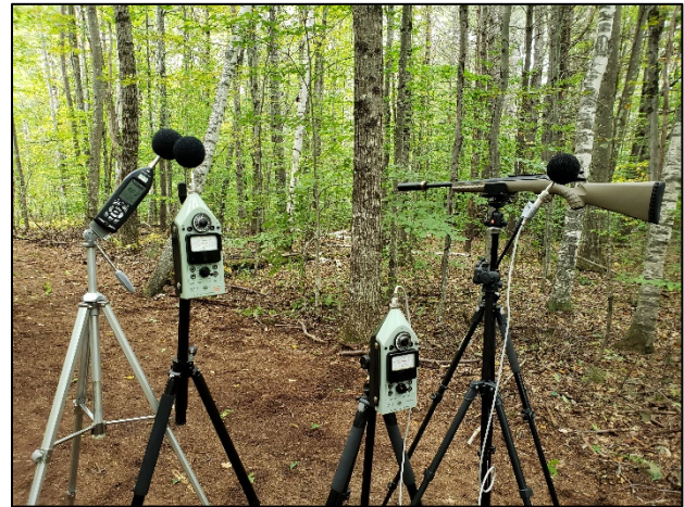
Photo 1: Equipment set up per MIL-STD 1474D
