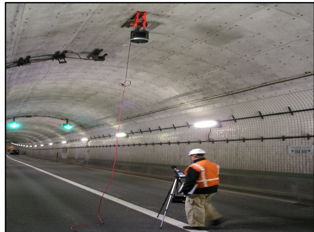
Photo 6. RSS Noise Measurements (Site 1)
