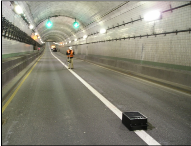
Photo 7. Reverberation Time Test (Site 5)
