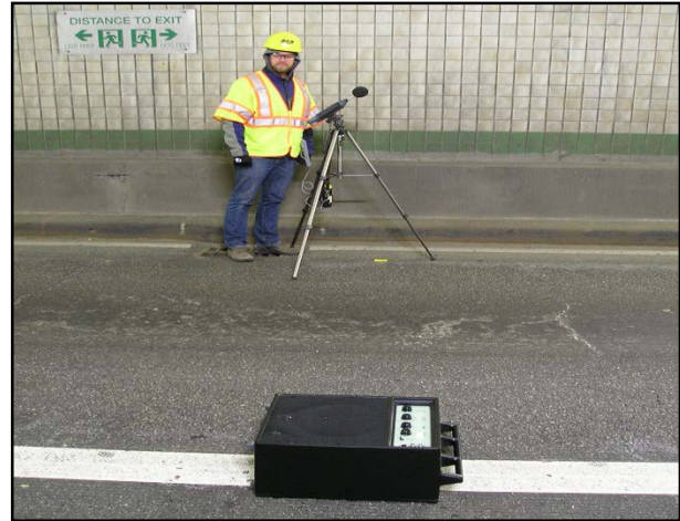
Photo 8. Reverberation Time Test (Site 2)
