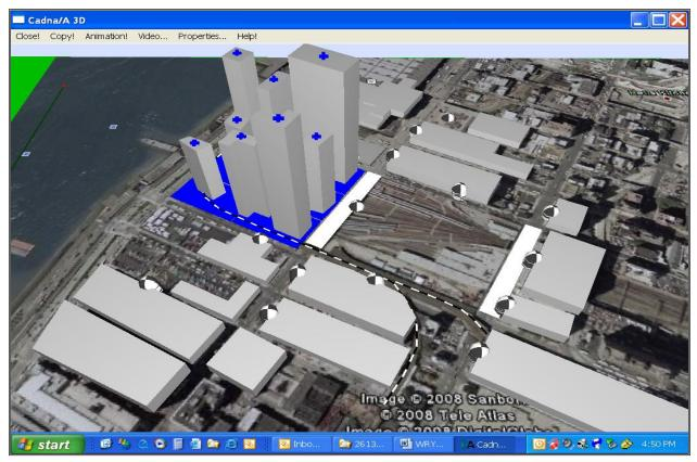
Figure 2. Cadna-A model input (typical) for the Western Rail Yard project
