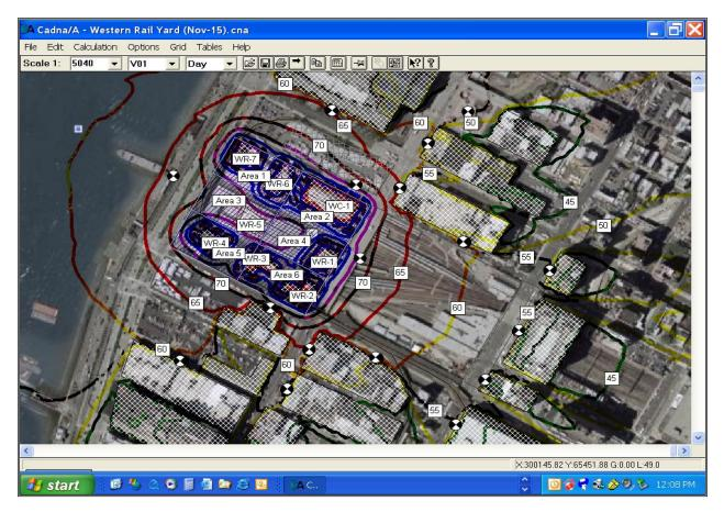
Figure 3. Cadna-A model output (typical) for the Western Rail Yard project
