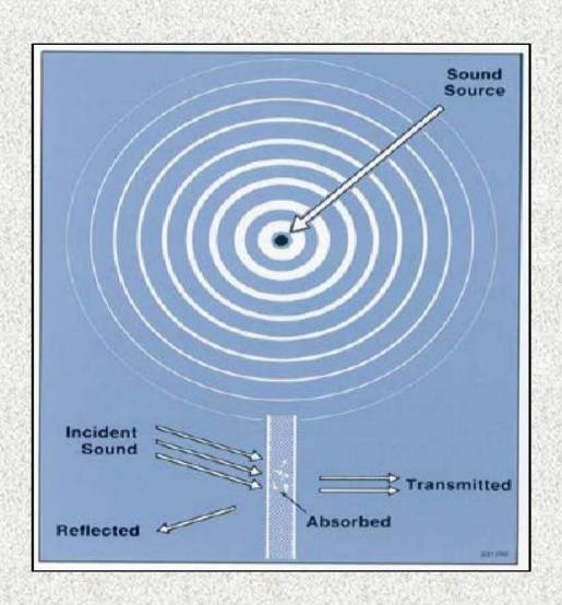
Acoustic Point Source in Free Field with Spherical Divergence:
